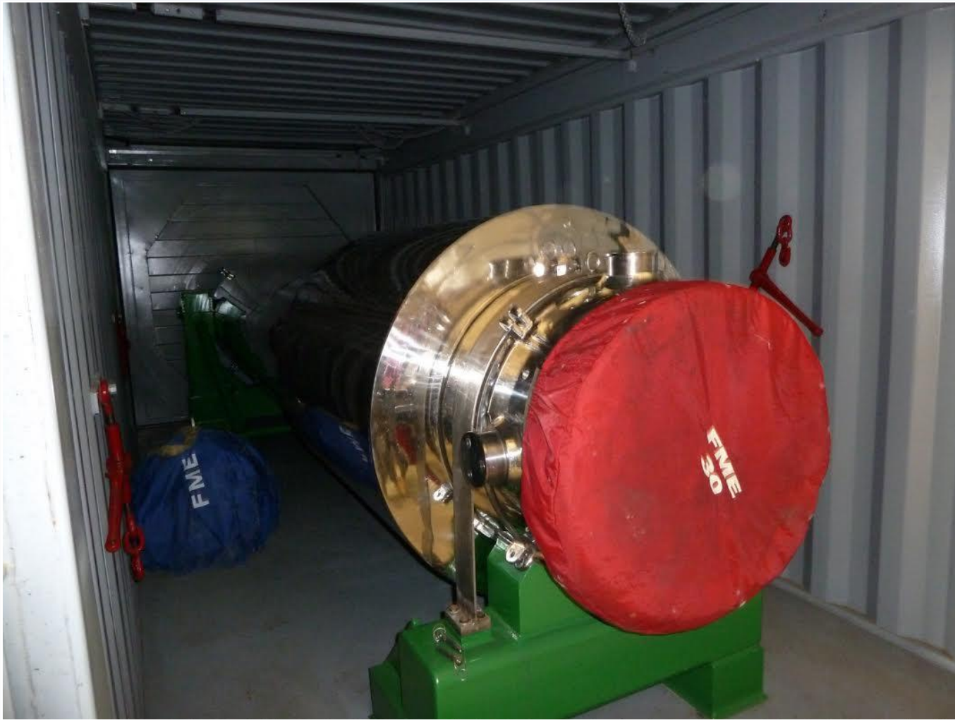
NAC-LWT loaded for transport. Not shown are the impact limiters that cover the two ends (the top and the bottom of the cask)
