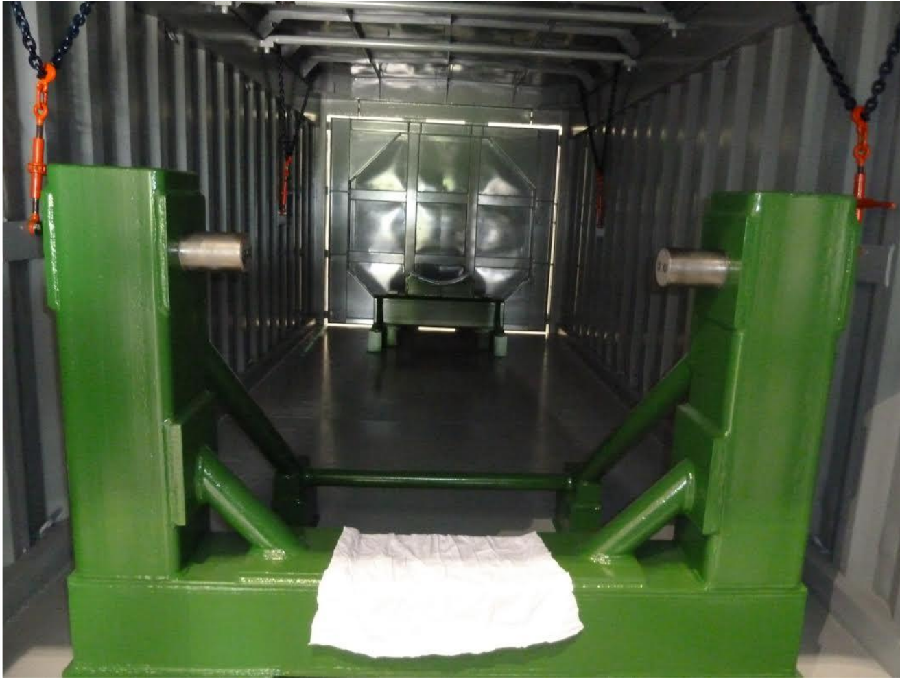
The inside of the NAC-LWT ISO container showing the substantial cradle that holds the cask.
