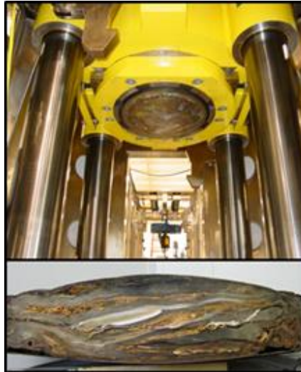
The waste drum supercompactor at AMWTP exerts 4 million pounds of force. This helps reduce the number of shipments and maximizes disposal space in WIPP
