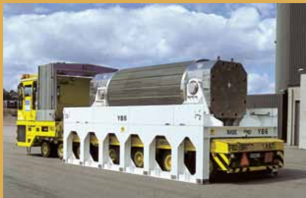
A preferred practice today is to place sufficiently cooled used nuclear fuel in physically robust steel and concrete casks that can be stored either vertically or inserted horizontally into reinforced concrete bunkers.
