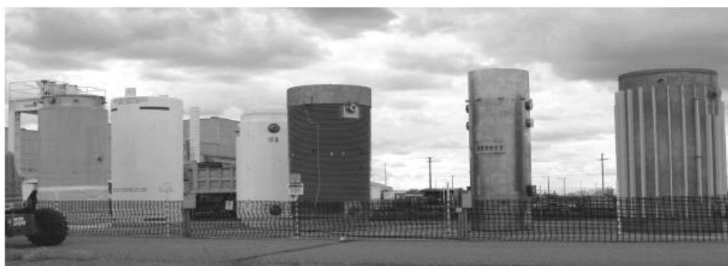
Figure 2. Commercial Dry Storage casks used in SNF tests at the INL Left to Right: REA 2023; VSC-17; TN 24P; V21; 125B; MC-10
