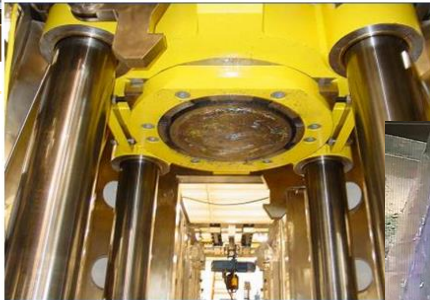
The Supercompactor used to treat transuranic waste at AMWTP (above) is nearing the end of its mission.
