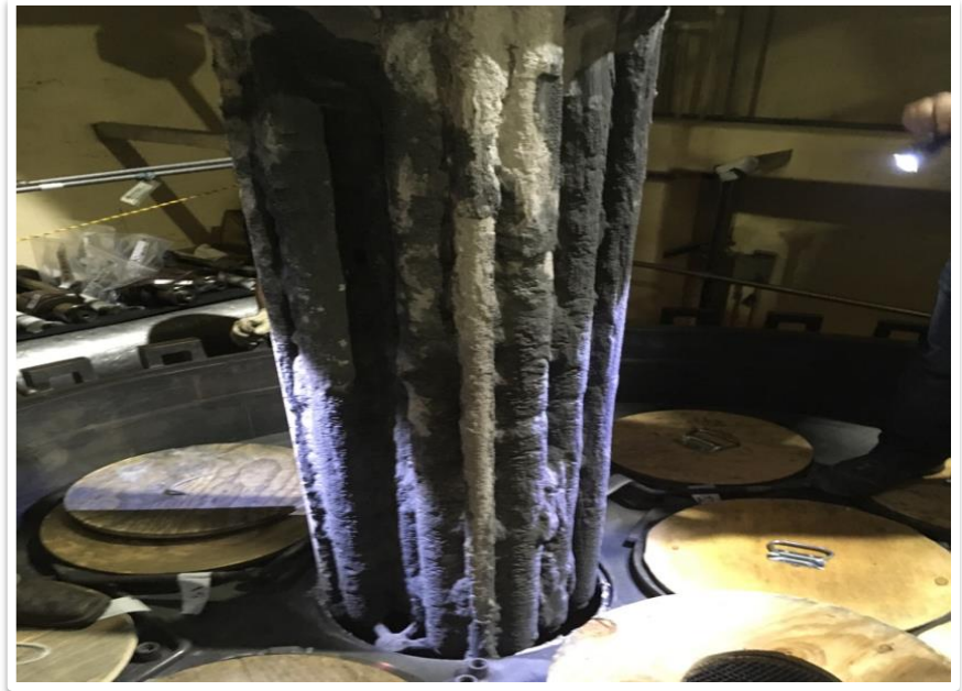
Seeking solutions to clogging of PGF filters.
