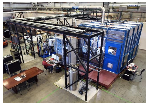
High Temperature Steam Electrolysis Test Platform
