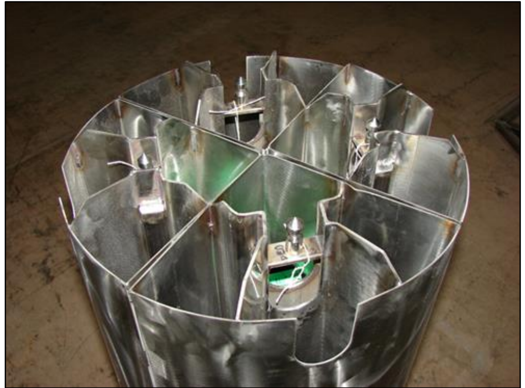
New four bucket storage design for placement of 16 ATR SNF elements into the CPP-603 storage canister.
