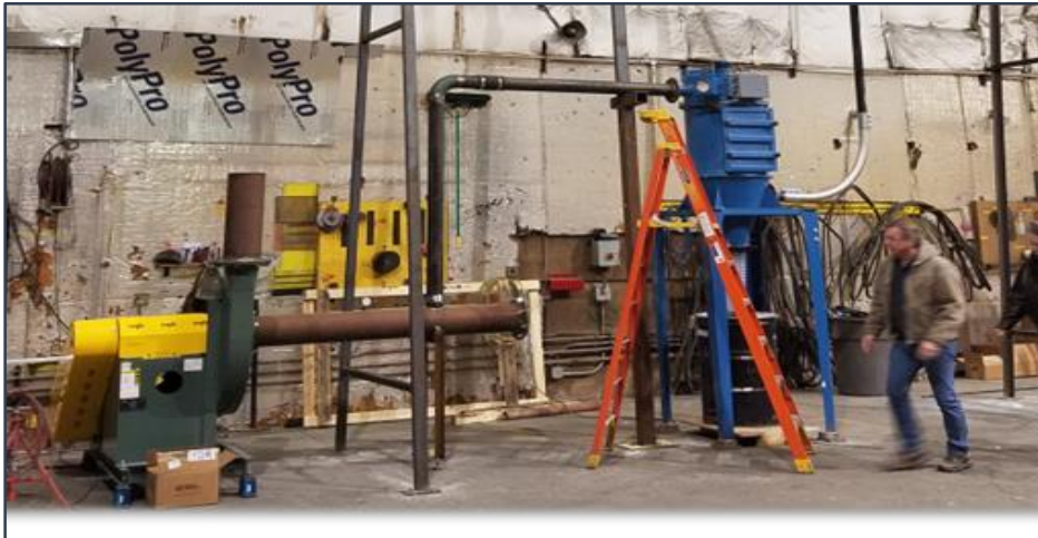
Full scale mockup of dry de-con system
