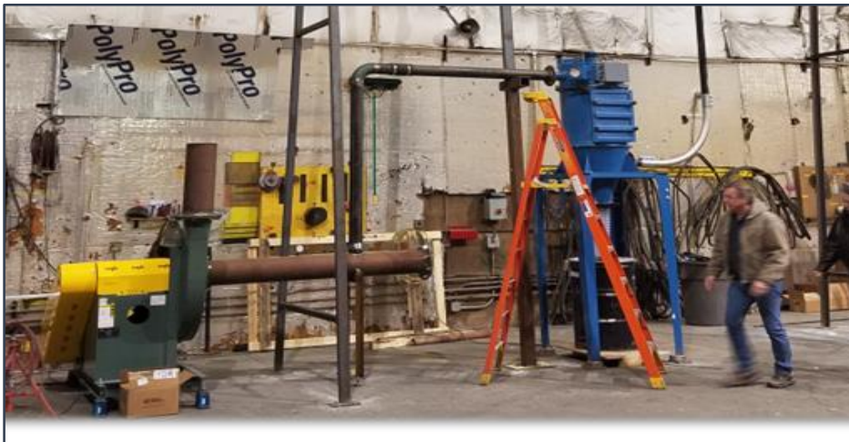
Full scale mockup of dry de-con system
