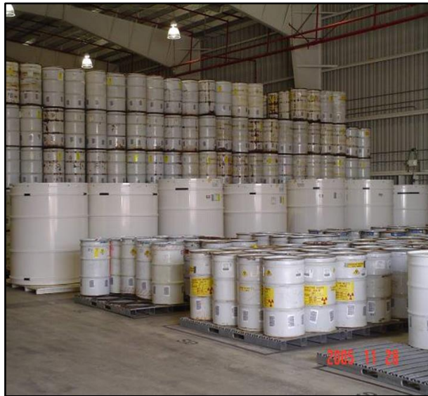
Contact-handled TRU waste in storage awaiting shipment to WIPP
