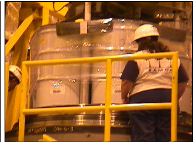
CH TRU waste being loaded into a TRUPACT II for shipment to WIPP
