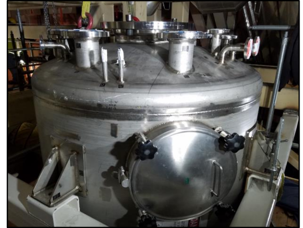
ASME conditioning tank hanging in the 4-Pack
