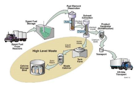
Fig 3. Spent Nuclear Fuel to Calcine Process Source: [18].
