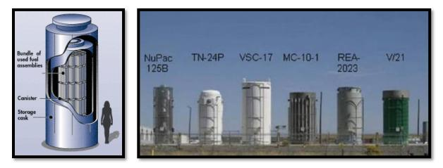
Fig 3 and 4. Example of dry cask storage. Source: [18] (Left); [22] (Right).
