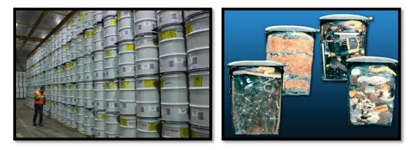
**Fig 4.** TRU waste in white 55-gal steel drums that are certified and ready to ship to the WIPP (*left*), *Source:* [21]. Simulated waste inside steel drums (*right*), *Source:* [22].
