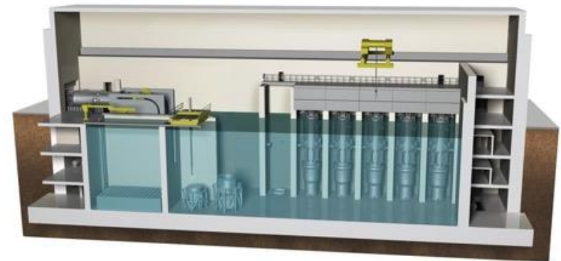
Cut away of NuScale small modular reactor (SMR)
