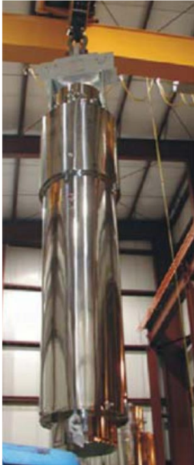
NAC-LWT cask held with the crane in HFEF high bay during qualification efforts
