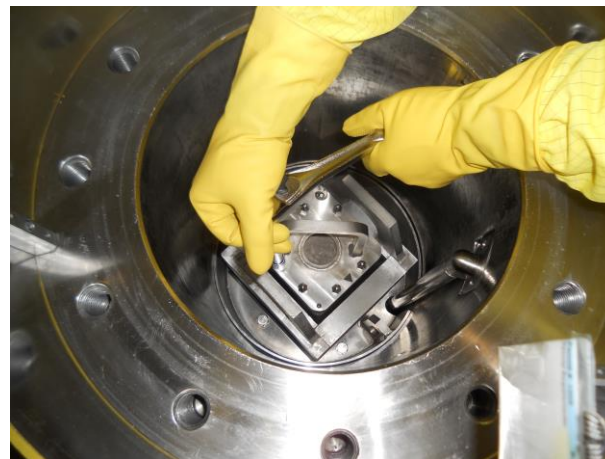
Shipping container where rods are loaded within the NAC-LWT cavity
