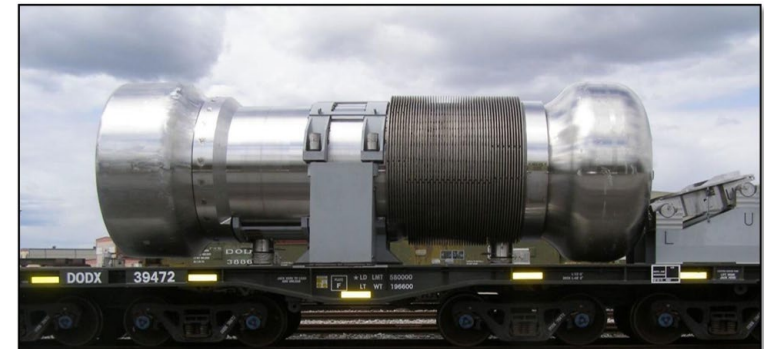
M-290: Aircraft Carrier spent fuel shipping container
