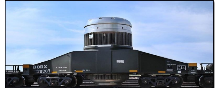
M-140: Submarine spent fuel shipping container
