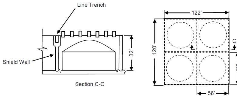
**Fig 4.** Diagram of square vaults containing SBW tanks WM-187, WM-188, WM-189, and WM-190.
