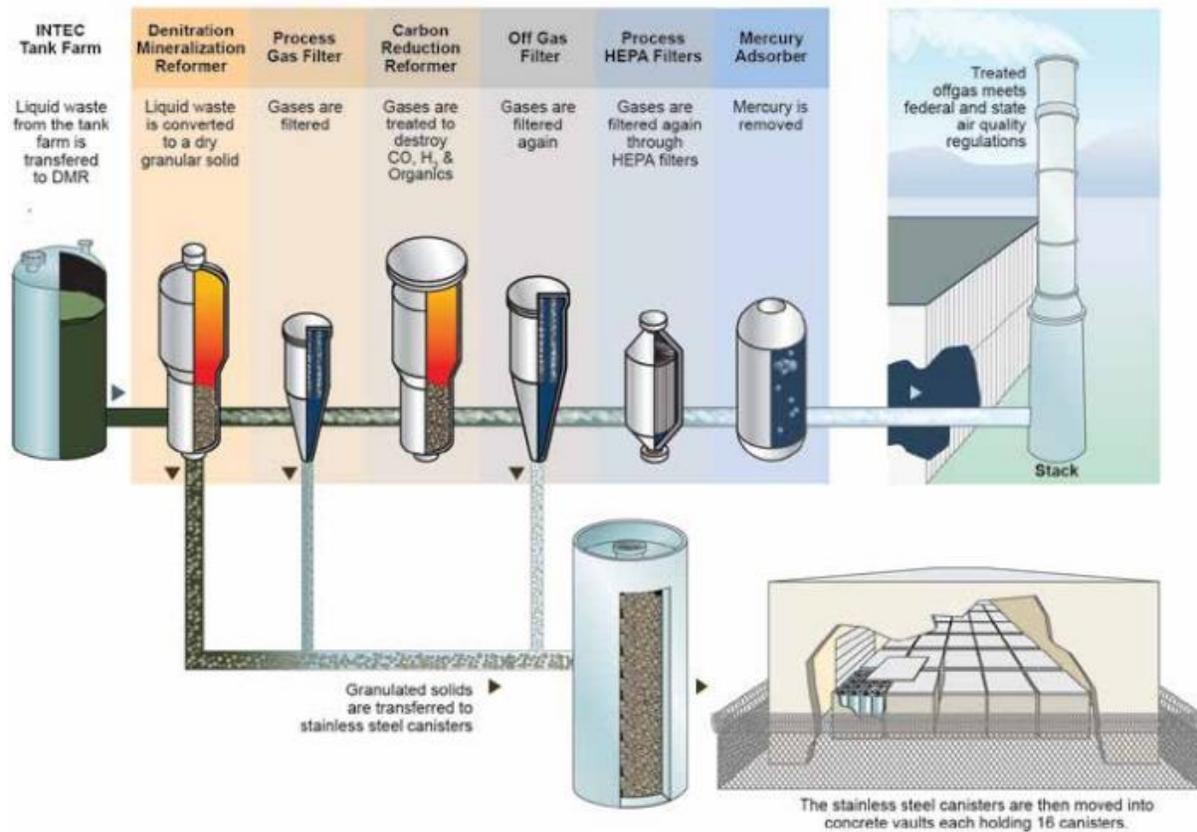
**Fig 5.** Simplified Integrated Waste Treatment Unit (IWTU) process flow. *Source: [11].*
