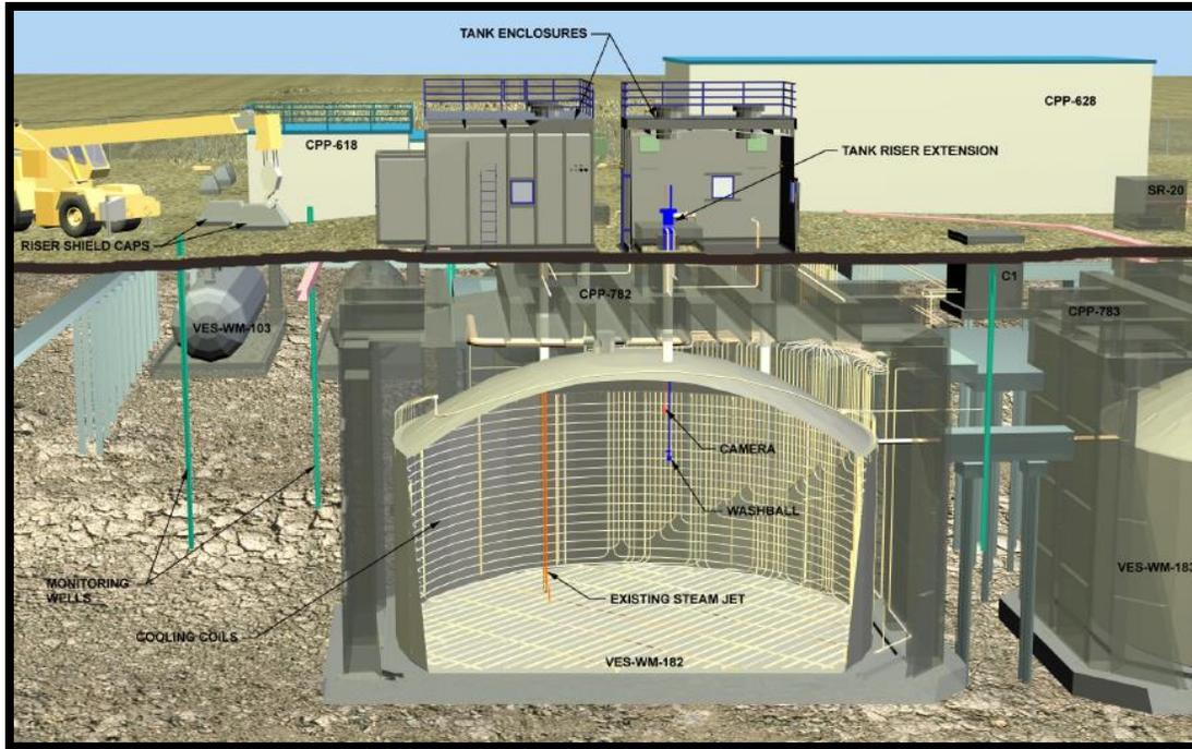
Fig 2. INTEC Tank Farm Facility tank WM-182 side view. Source: [14].
