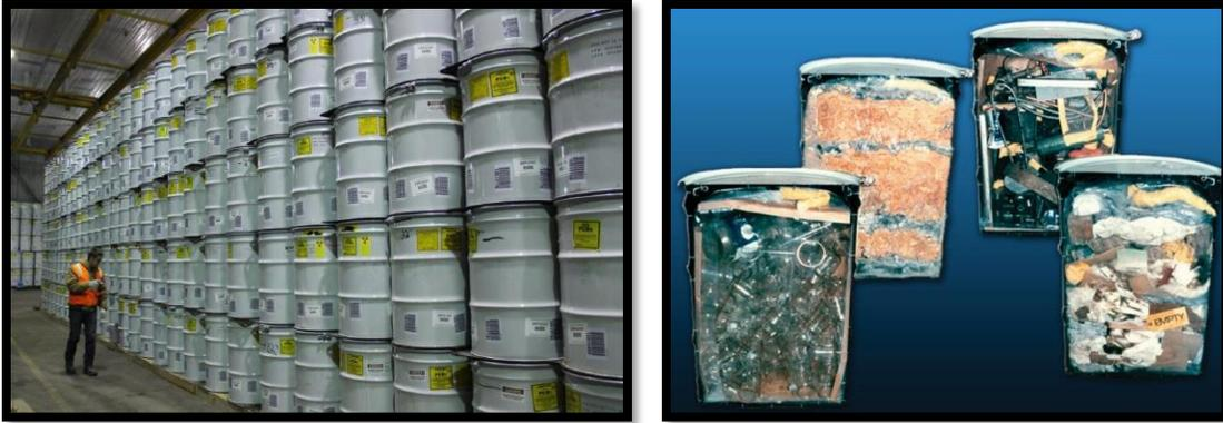
**Fig 4.** TRU waste in white 55-gal steel drums that are certified and ready to ship to the WIPP (*left*), *Source: [21]*. Simulated waste inside steel drums (*right*), *Source: [22]*.
